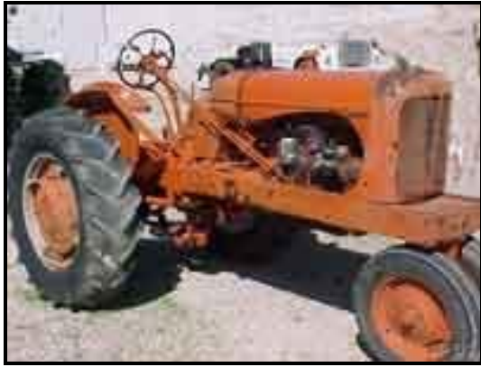
FIGURE 3.2: Tractor without a roll-over protective structure
