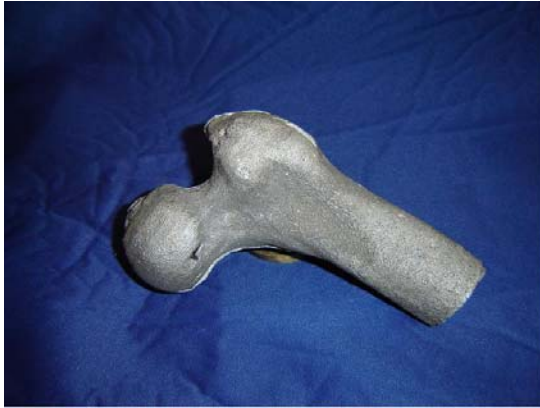
Fig. 7: Aluminium casting made through direct casting into the sand mould cavity
