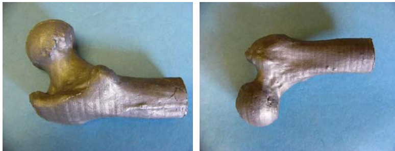
Fig. 8: Stainless steel casting generated through investment casting of parts grown in Prime Cast 100
