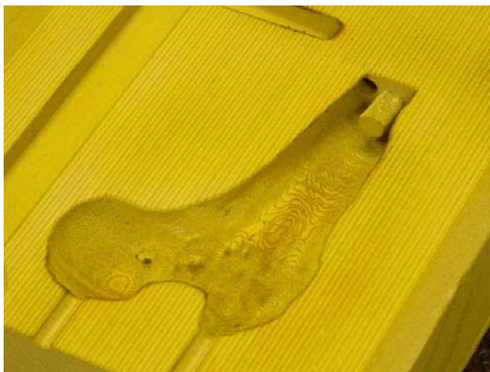
Fig. 6 : Sand mould grown on EOS S700
