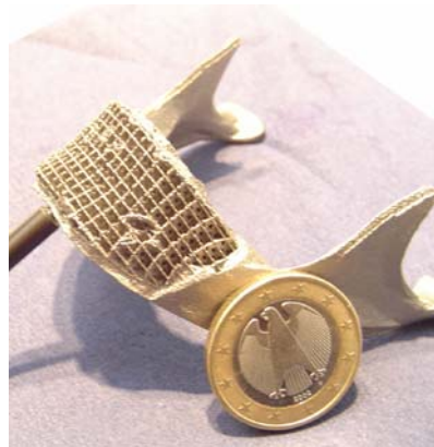
Fig 12: Titanium implants grown by SLM
