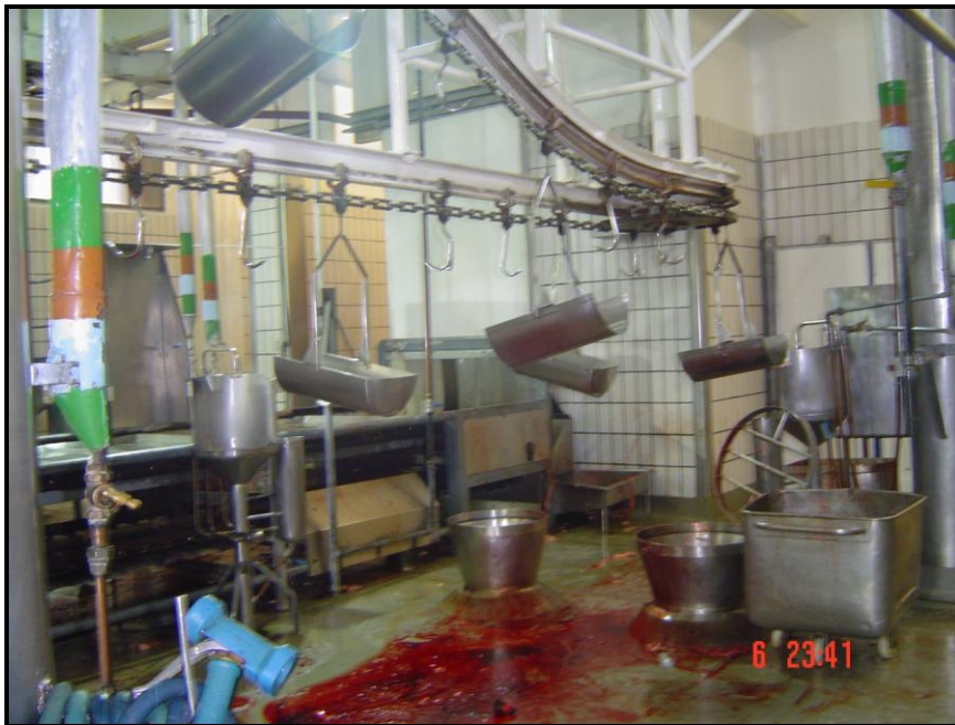
Figure 2.6: The conveyor system, trolley and conveyor shafts used to transport offal from one station to another for further processing
