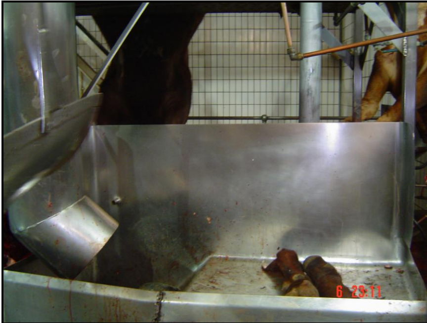
Figure 2.8: Feet thrown into the conveyor shaft
