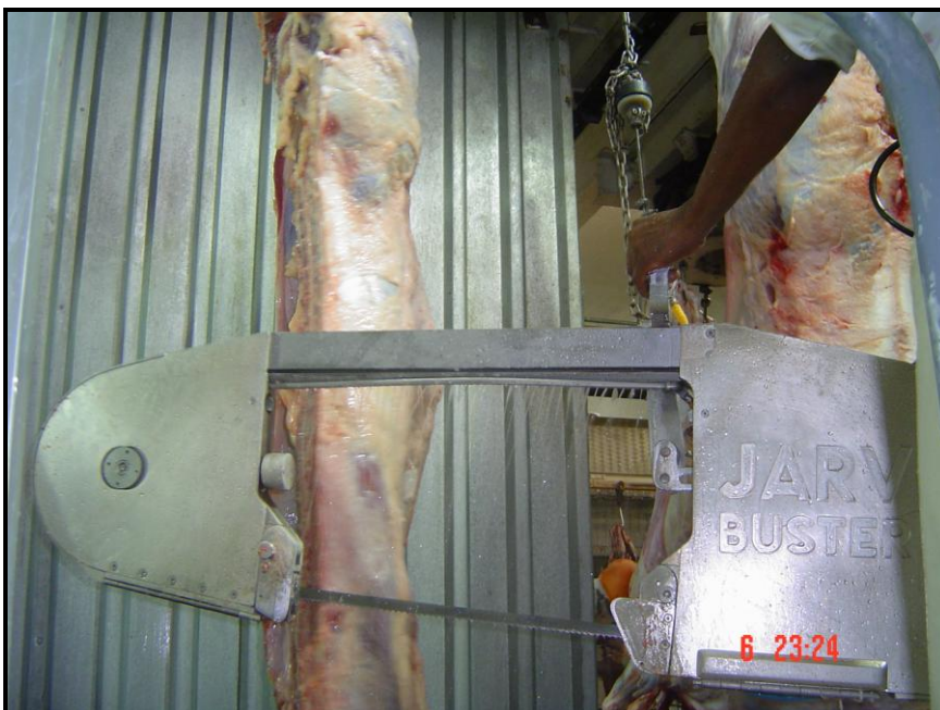
Figure 2.11: Carcass-splitting saw used to divide the carcass into two parts
