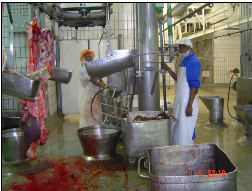
Figure 2.5: Wall, floor and equipment as sound-reflecting surfaces on the slaughter floor
