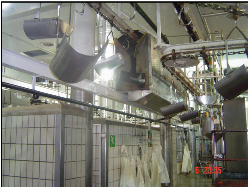
Figure 2.3: Fittings and equipment used on the slaughter floor as sound-reflecting surfaces on the slaughter floor
