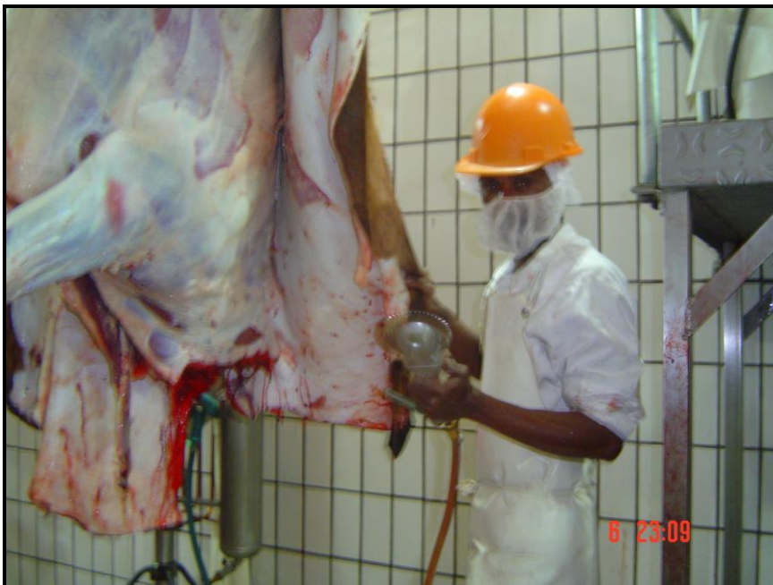
Figure 2.9: An employee using circular saw blade to de-skin a cattle carcass
