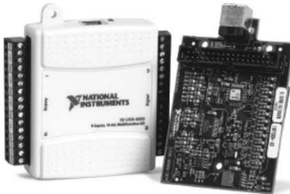
Figure 13: NI USB-6009 inside and outside an enclosure
