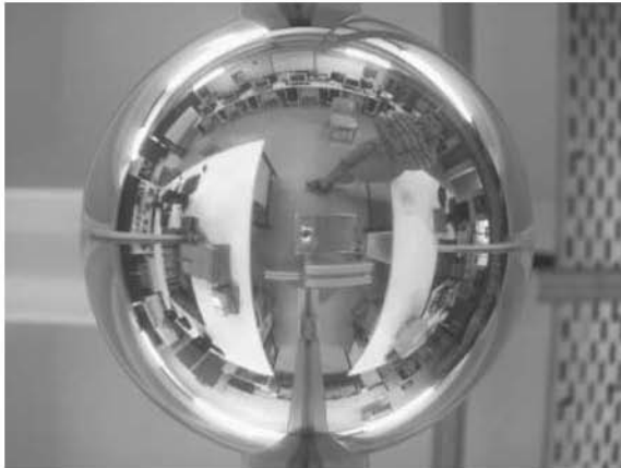
Figure 3 : Dome mirror picture before conversion into panoramic format
