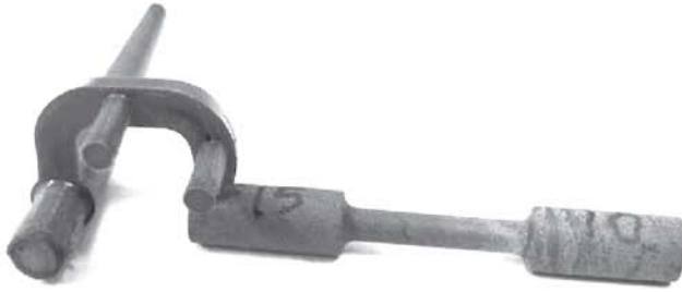
Figure 6: Photograph of the green specimen and feeding system
