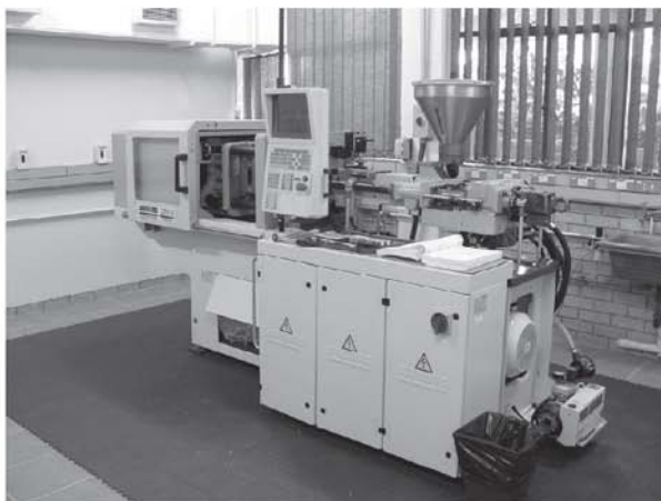
Figure 5: Photo of the MIM Injection moulding machine
