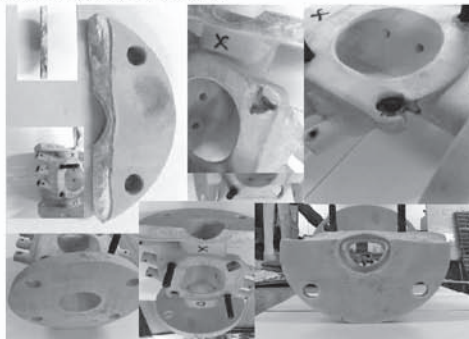
Figure 6: Collage of pictures showing the damaged Z-Corp infiltrated diaphragm valve
