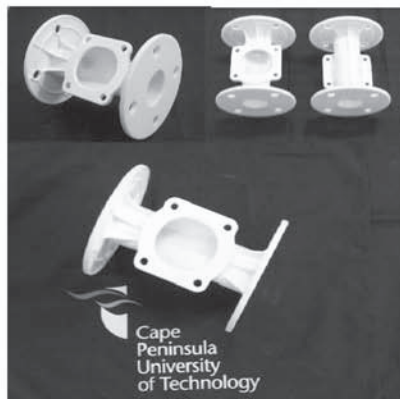
Figure 16: A collage of pictures showing the wax infiltrated Z-Corp starch printed patterns
