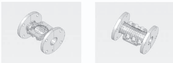
Figure 3 a & b: CAD model of the reverse engineered diaphragm valve
