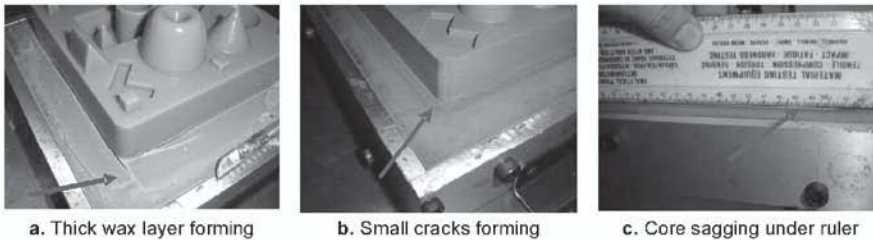
Figure 7: Polyamide core compressing
