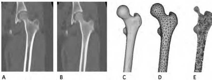
Figure 1: Sequential steps to produce image-based volumetric meshes for FEA of a human femur; coronal CT slice (A), segmentation of the femur (B), the reconstructed 3D model (C), the optimized surface mesh (D) and a section through the volumetric mesh with colour-coded material properties (E).
