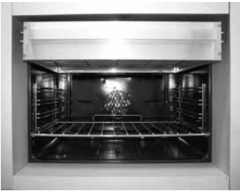
Figure 2: Experimental hybrid IR-convective dryer
