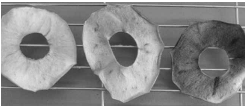
Figure 9: The result of drying samples to lower moisture contents
