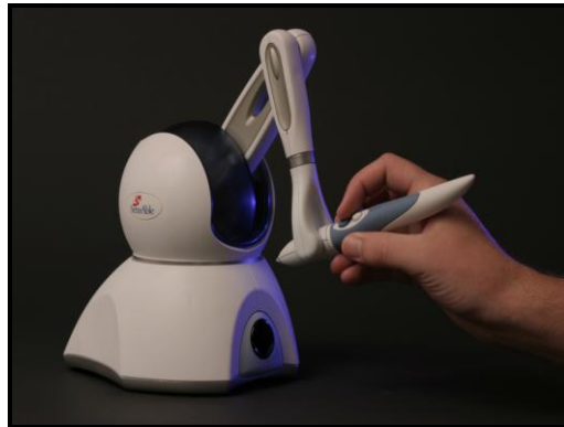
Figure 2. 1. Omni PHANToM haptic device, SensAble Technologies, 2007.
