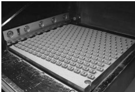
Figure 6. Case study work pieces in DMLS rapid manufacturing process
