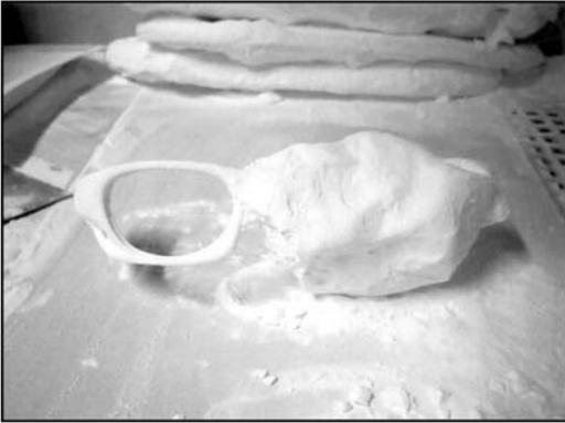
Figure 2: A frame immediately after the laser-sintering process.
