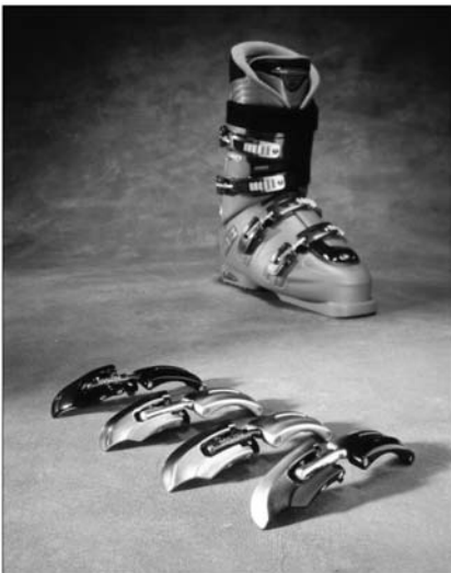
Figure 4: Ski boot buckles manufactured in polyamide by laser-sintering
