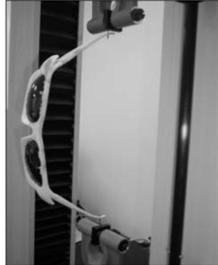
Figure 3: Example of quality control – mechanical testing.
