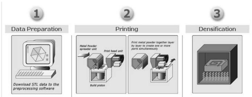
Figure 9: Three-step process for ProMetal 3D Printing [11]
