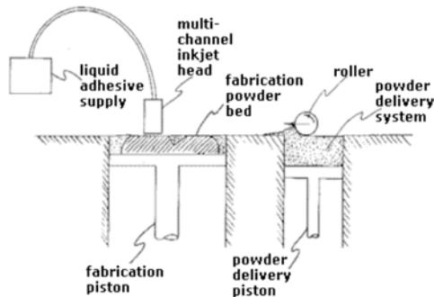
Figure 7: Schematic diagram of 3D Printing – Drop-on-Bed [6]
