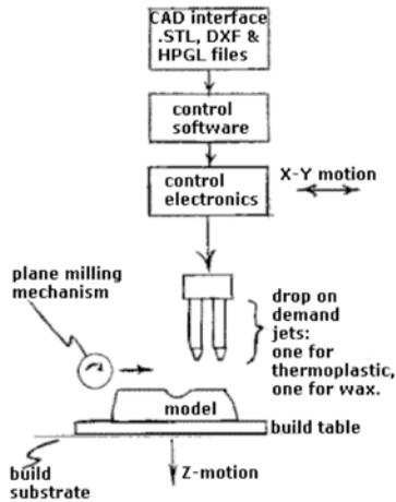
Figure 2: Schematic diagram of 3D Plotting [6]
