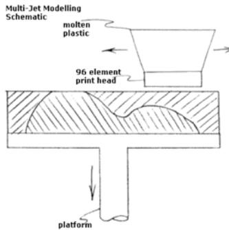
Figure 4: Schematic diagram of Multi-Jet Modelling [6]
