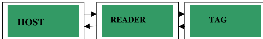
Figure 1: This is the block diagram of the RFID system. The reader acts as an interface between the host and the tag.
