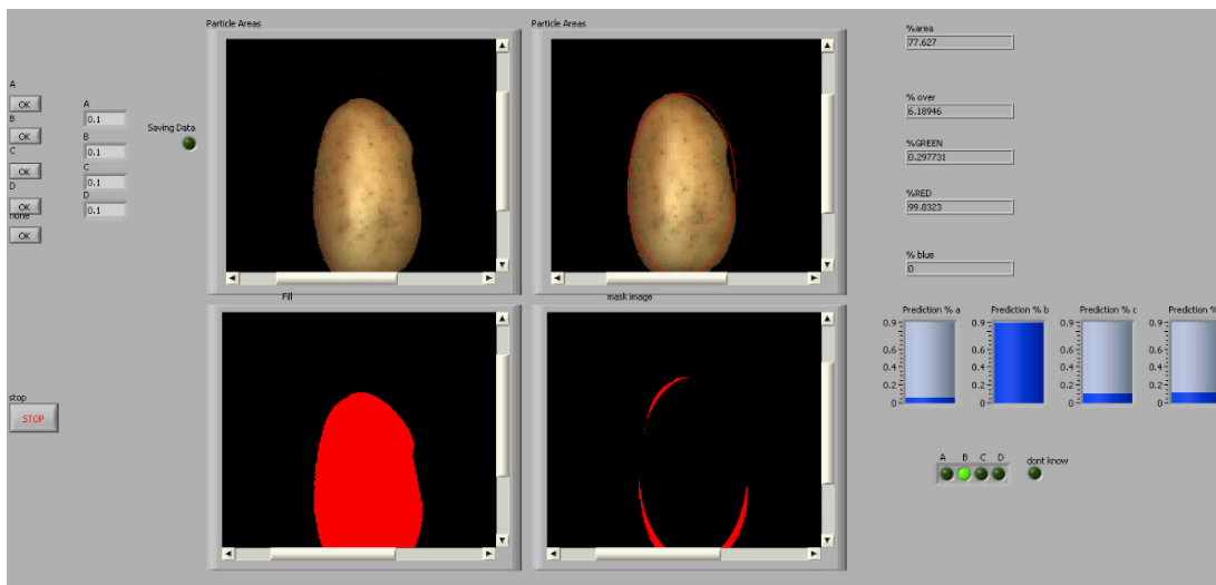
Figure 6-22: The artificial intelligence machine vision grading system front panel with a large potato under the camera sorting it to option B
