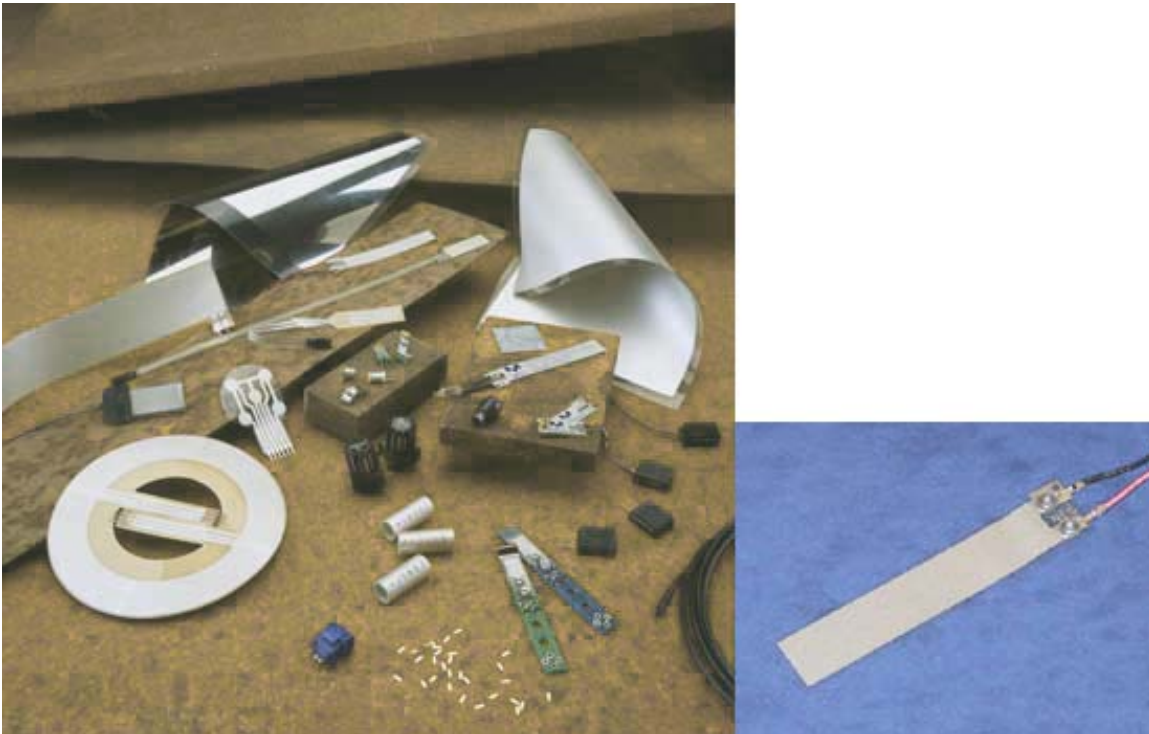
Figure 3.5 Piezoelectric films on the market (left); example of the piezoelectric film used in this research (right).
