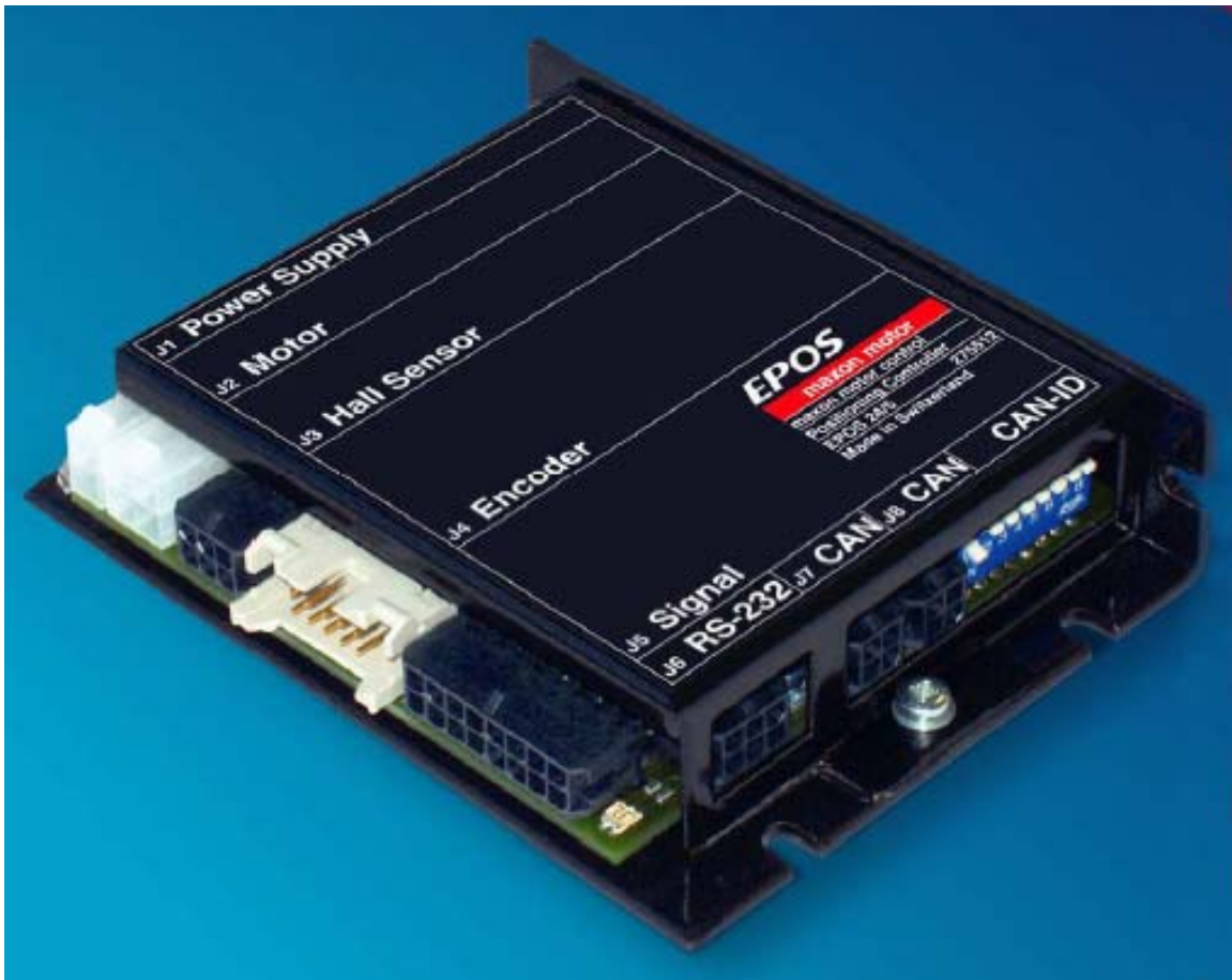
Figure 3.14 Maxon Epos 24/5 5A DC motor-positioning controller used to control the gripper motor interfaced with LabView™.
