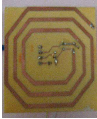
Figure 3.19: Antenna constructed using the Roland Modela MDX-20
