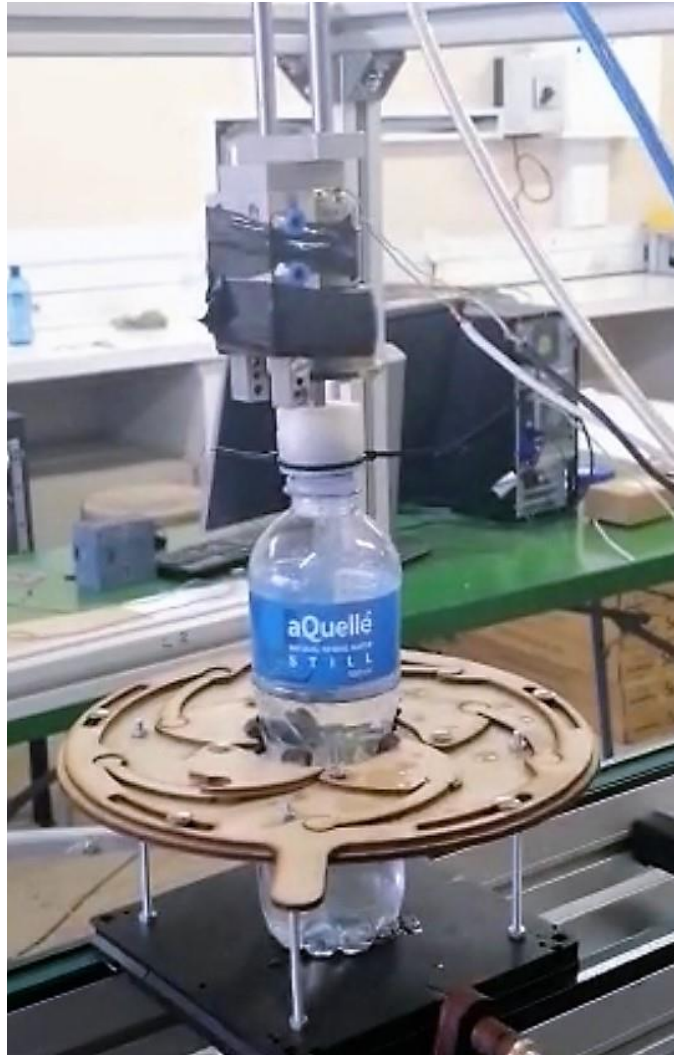
Figure E.3. A water bottle being capped at SMU2.
