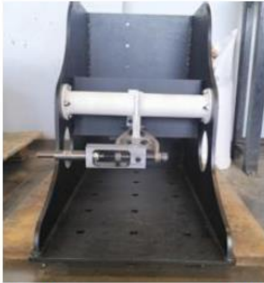
Figure 3: Test jig with the scale-down nose wheel fork of the AHRLAC aircraft.
