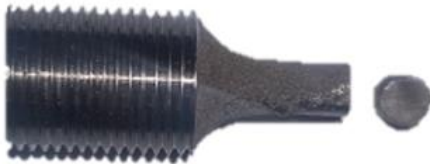
Figure 3.6: Illustration of the cross sections cut on HCF test specimens using an AU-500 iA Accutex wire-cutting machine
