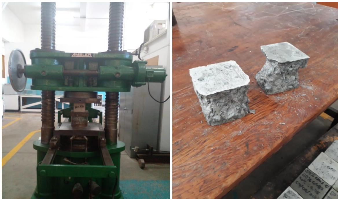
Figure 3-9: Photograph showing the positioning of concrete specimens on the AMSLER machine and their definition of failure after compression
