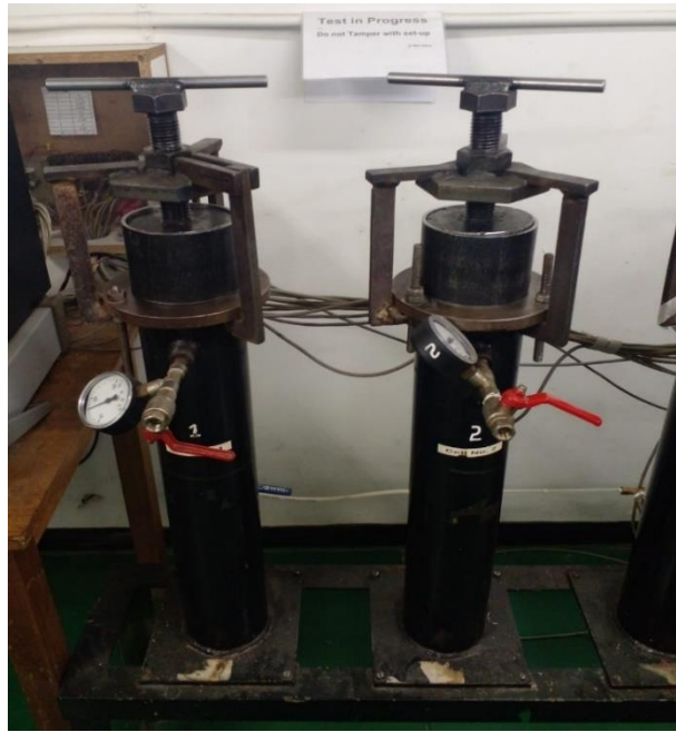
Figure 3-12: Photograph of oxygen permeability test set-up
