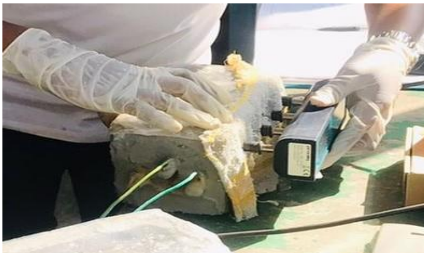
Figure 3-18: Photograph of resistivity measurements with the four-point Wenner probe
