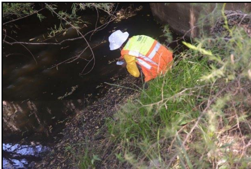
Figure 3.9 In situ dissolved oxygen measurement at Mooi River before the Potchefstroom wastewater treatment works
