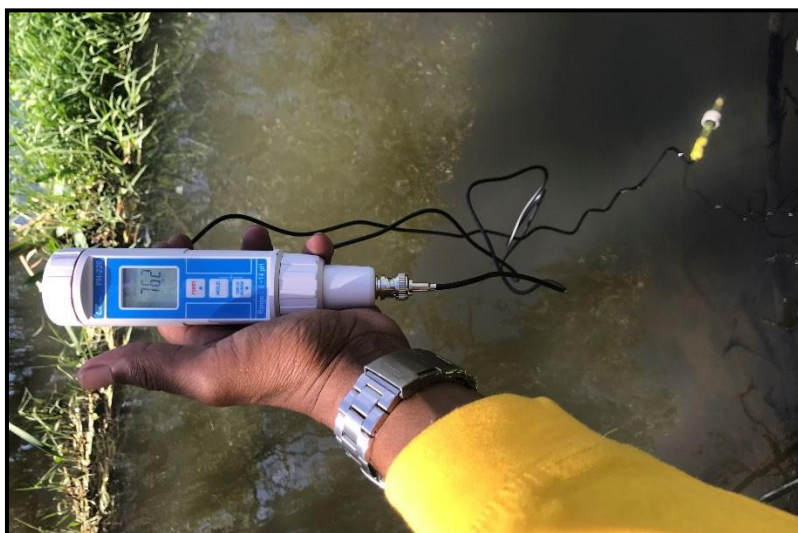
Figure 3.6 Field measurement of pH using a pH meter
