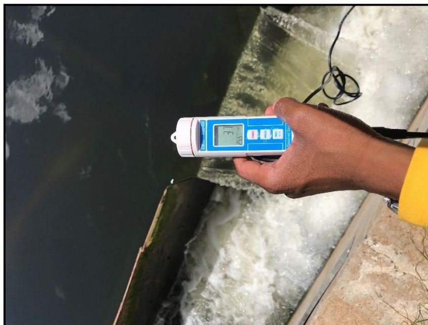
Figure 3.7 Field measurement of dissolved oxygen and temperature using a dissolved oxygen meter
