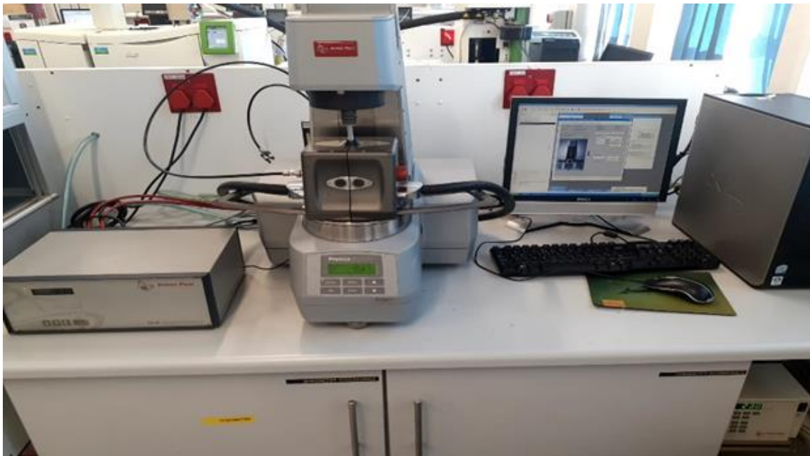
Figure 3.6 The equipment that was utilized to determine the dynamic rheological measurements.
