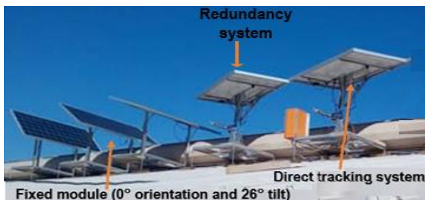
Figure 4.1. The practical system with the PV modules used for calibration.
