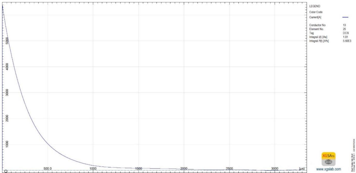
Figure V: Boet Troskie Hall building 8 th down-conductor current distribution
