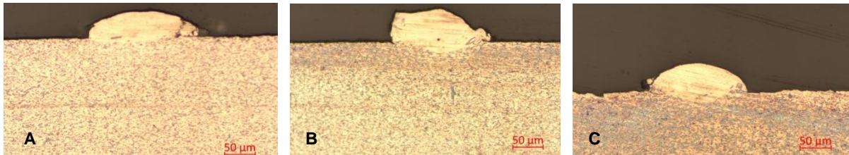
Figure 58. Cross-sectional view of single laser tracks at a laser power of 350 W (A) 2.8m/s (B) 3m/s (C) 3.4m/s
