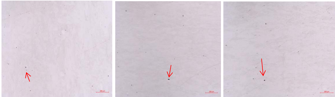
Figure 84. Optical microscope pictures of Ti6Al 3D part (a) Top view (b) Side view (c) Front view un-etched.
