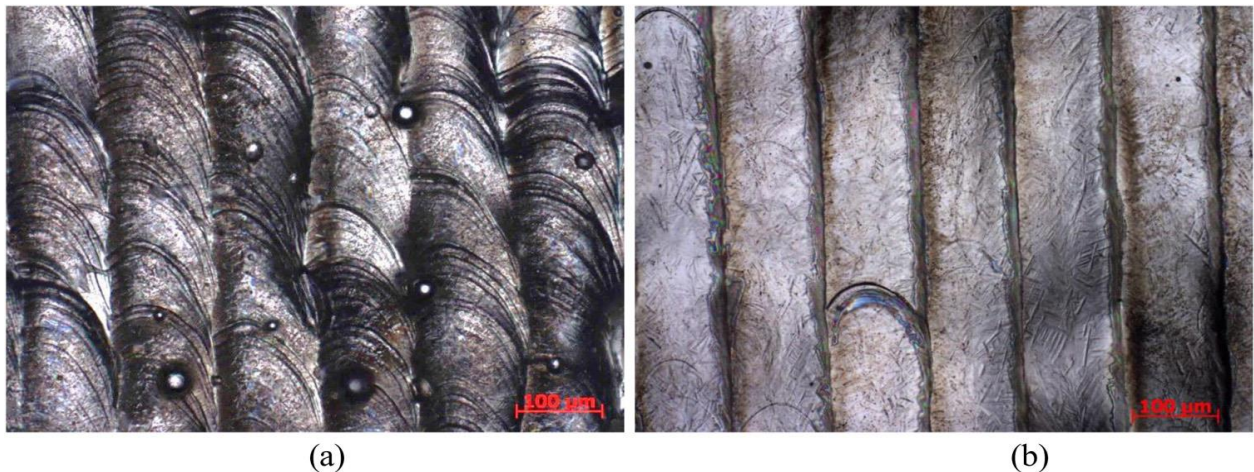
Figure 19.(a) Top view of single layer produced by one-zone strategy (b) and two-zone strategy (Yadroitsev et al. , 2015).
