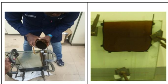
Figure 2: Pouring of the mixed reinforced coconut shell powder composite into a mould and a cast CSP epoxy resin/coconut particle composite
