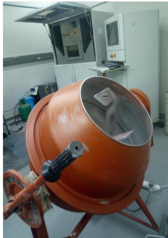
Fig. 7. A concrete mixer used at CRPM.
