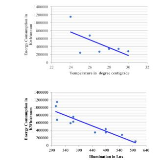
Figure 2. Relationship between indoor temperature and energy consumption
