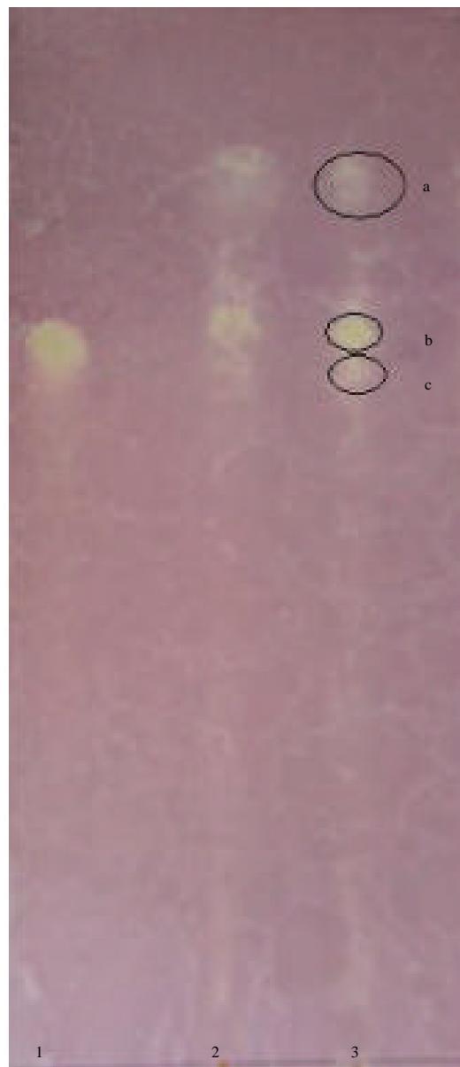
Fig. 1: Chromatogram of gallic acid (1) and A. laricinus aqueous extract (2 and 3), separated with methanol:chloroform: hexane (70:20:10%) and sprayed with DPPPH. The yellow spots indicated antioxidant activity (RF values: a = 0.87; b = 0.38; c = 0.35)
