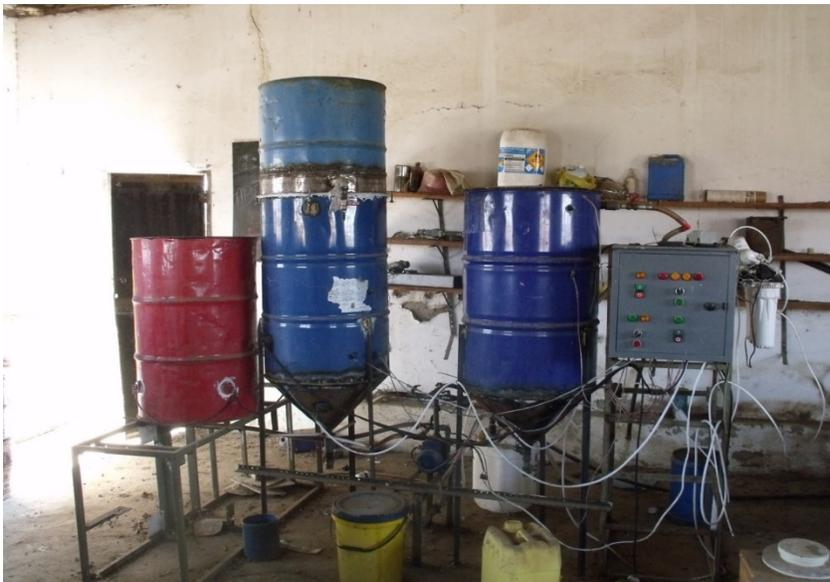
**Figure 5.4: Biodiesel production plant**
