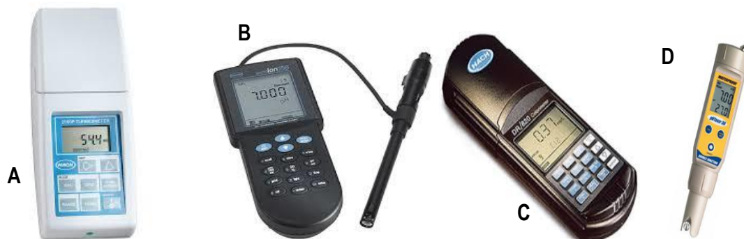
Figure 3.4 Hach instruments. A. 2100P turbidity meter. B. conductivity meter. C. DR/820 colorimeter. D. pH meter.
