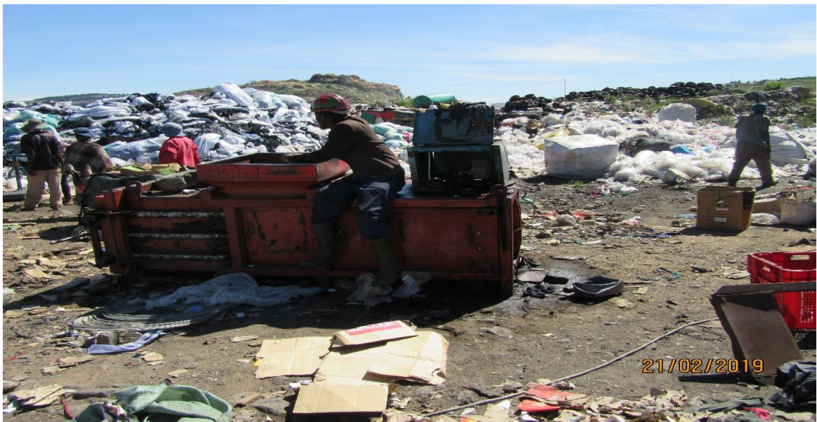
Figure 3.12: On-site diesel driven waste compacting machinery at the Mokota-koti dumpsite in the Maputsoe Urban Council area (Photograph: Motaung, 21 st February 2019).
