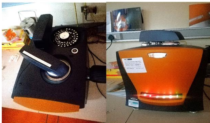
Figure 3.6: Top and front view of DSC instrument employed for analysing thermal properties.
