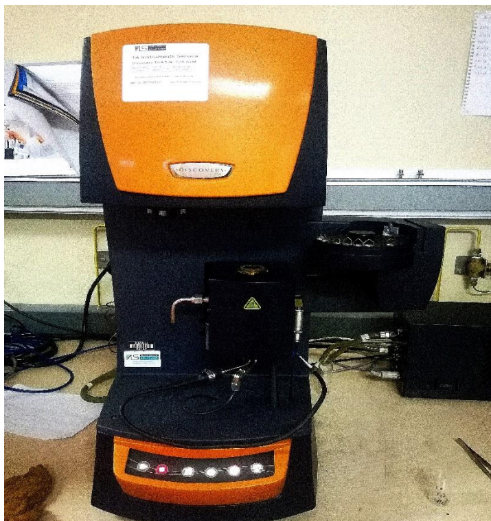
Figure 3.4: TGA instrument that was employed for analysing the thermal stability of the samples
