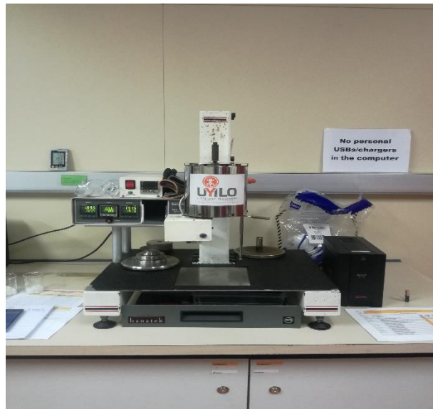
Figure 3.2: MFI instrument that was employed in this study for analysing the viscosity of the blends and blend composites
