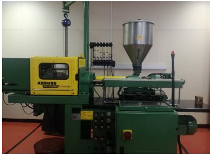
Figure 3.7: Injection moulding machine that was used for investigated samples
