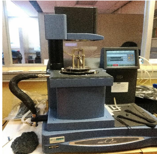
Figure 3.10: DMA instrument that was employed for analysing the thermomechanical properties of the blends and composites
