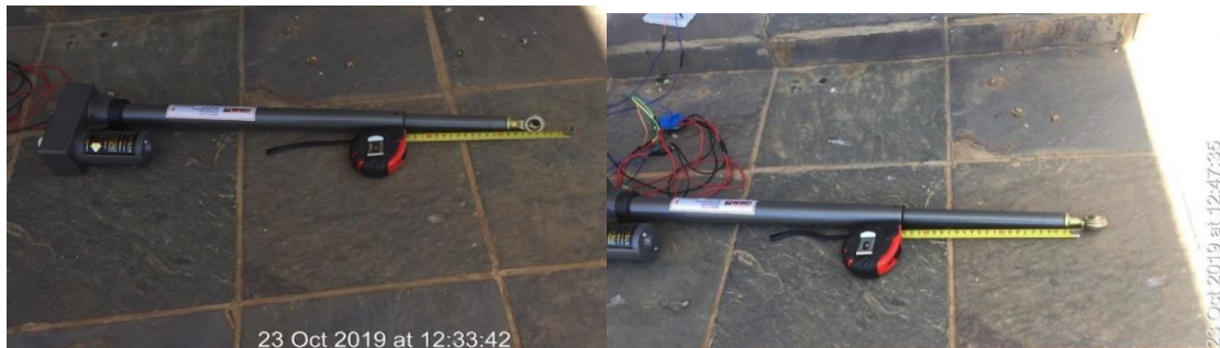
Figure 58: Actuator retracted and extended to achieve 20 degrees
