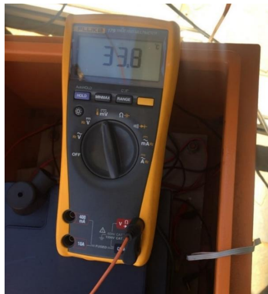
Figure 51: PV module surface temperature DMM reading
