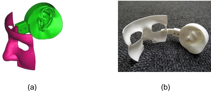
Figure 4.8 (a) Mask with orientation attachment. (b) Additively manufactured orientation guide
