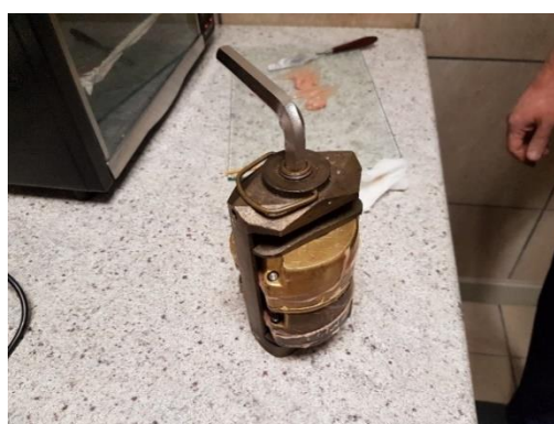
Figure 6.50 Flasks clamped tightly on top of each other.
