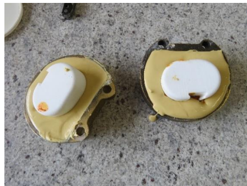
Figure 6.33 Bottom section of flask with moulds secured in plaster.
