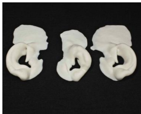
Figure 4.5 Additively manufactured copies of auricles.
