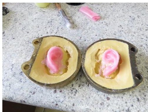
Figure 6.39 Bottom flask sections with wax patterns.
