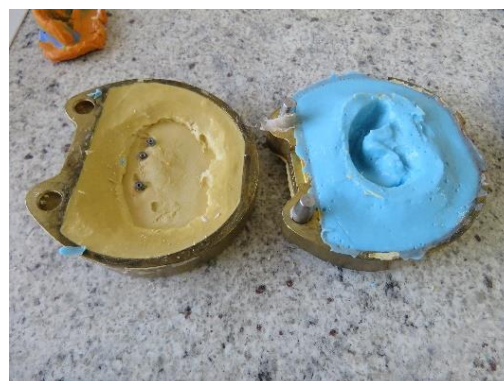
Figure 6.36 Bottom flask with implant positions and top flask with cavity.
