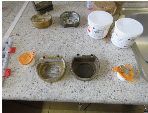
Figure 6.29 Moulds removed from guide rails.
