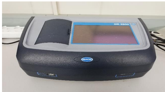
Figure 3.4 DR3900 spectrophotometer for the measurement of nitrate, ammonia, sulphate and total hardness.
