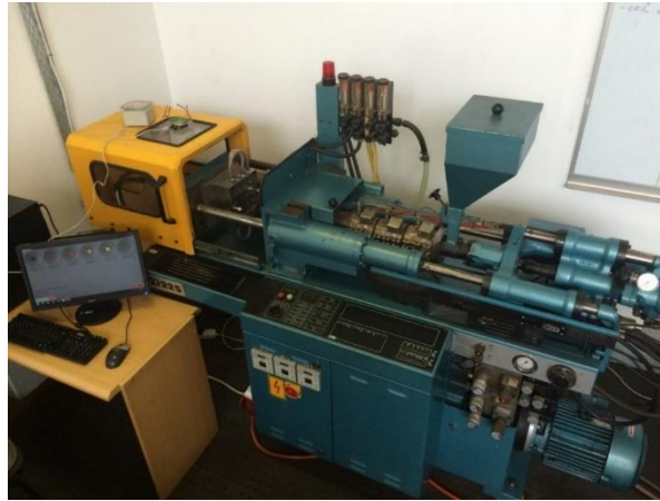
Figure 4.28: Dr Boy IM machine used during the IM trial with the PC interface used to record the temperatures of the mould.
