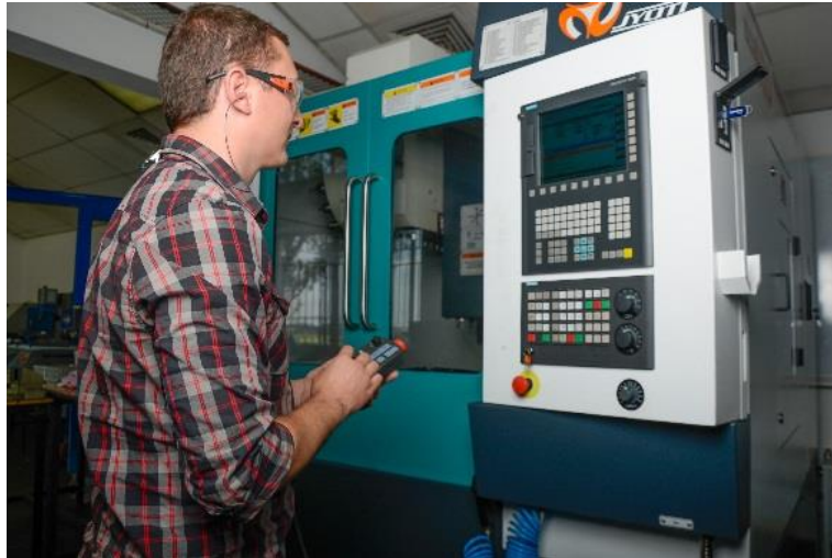
Figure 4.25: Jyoti VMC850 vertical CNC machine used to manufacture the mould components.
