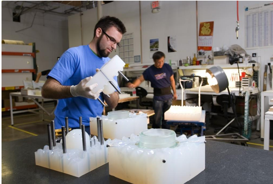
Figure 3.4: Assembly of a soft tool manufactured from silicon [51].
