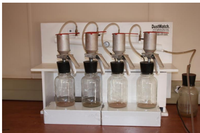
Figure 3.4 Fall-out dust vacuum filtering system with Buchner funnels.
