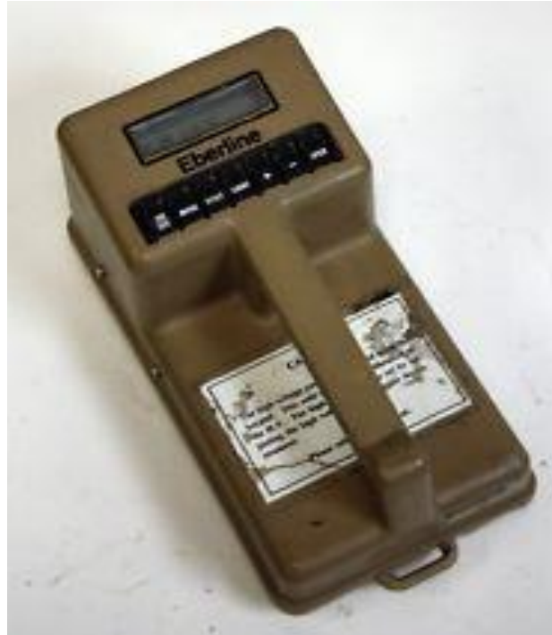
Figure 5.7: Eberline Smart Portable (ESP-2) data logging radiation survey counter
