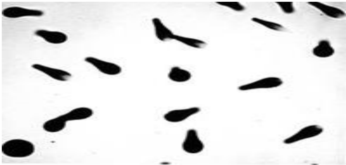
Figure 2.2: Nuclear tracks made visible by etching in concentrated hot NaOH (PARC RGM, 2018)
