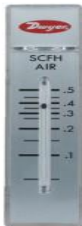
Figure 5.4: Dwyer air flow meter
