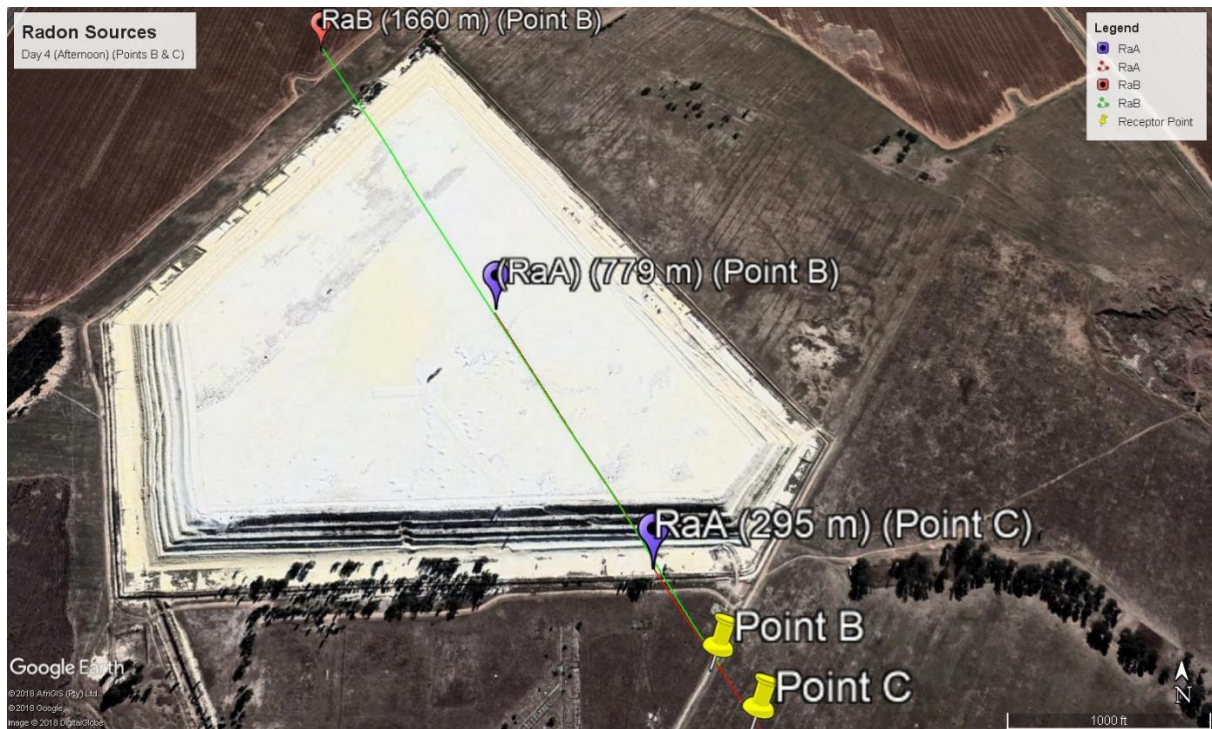
Figure 6.26: Day 4 afternoon radon source origins from back calculations (receptor points B and C).
