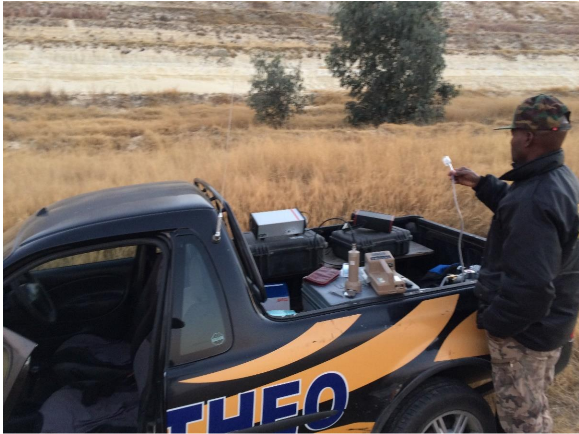
Figure 5.8: The setup used to deposit radon daughters on the filter paper.
