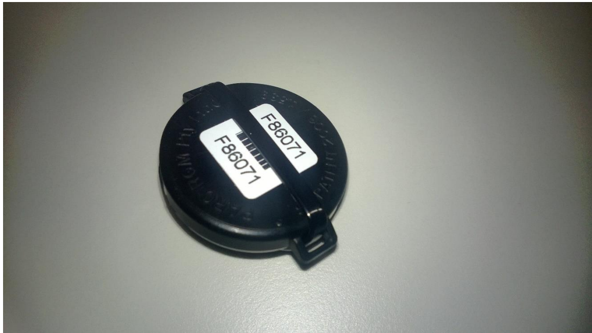
Figure 2.3: Radon Gas Monitor (RGM), a CR-39 based track detector (PARC RGM, 2018)
