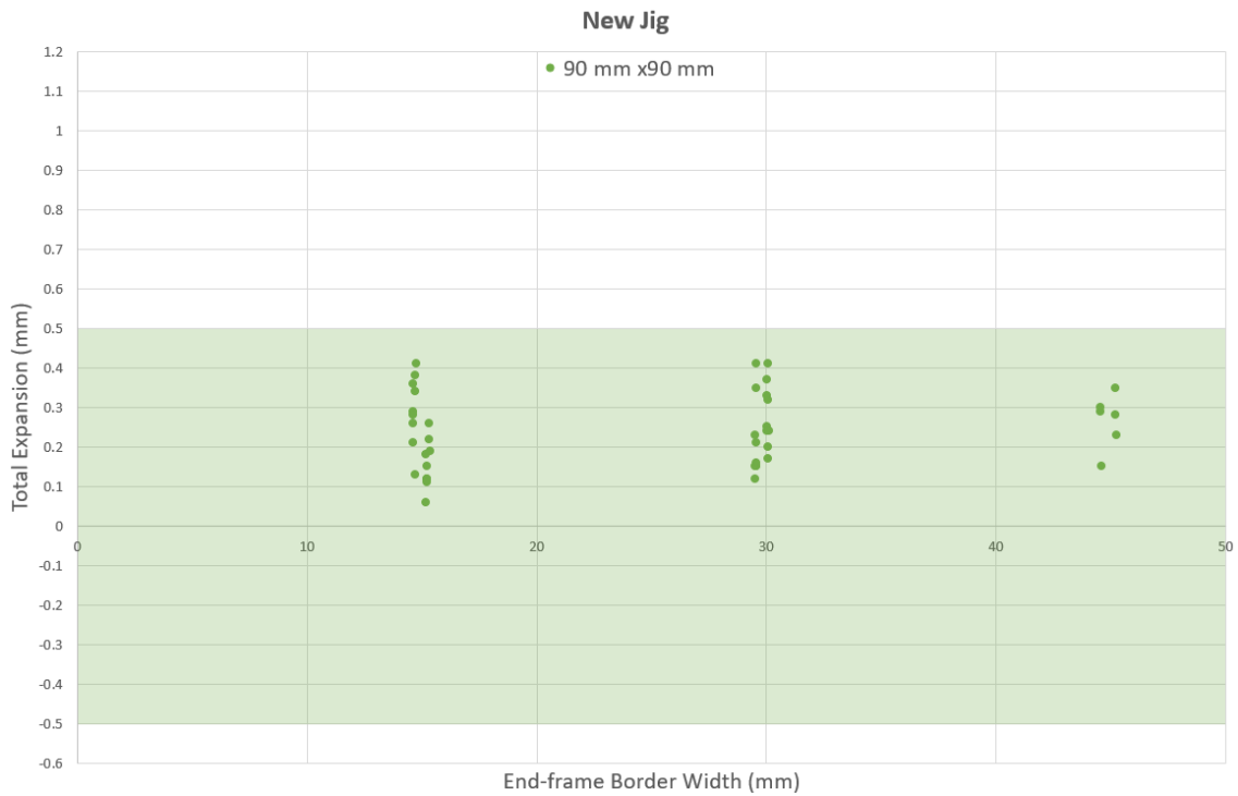
Figure 5.10: Total expansion vs end-frame border width for the 90 mm x 90 mm jig size. The average end-frame border widths are 15 mm, 30 mm and 45 mm which represent the solid cast
