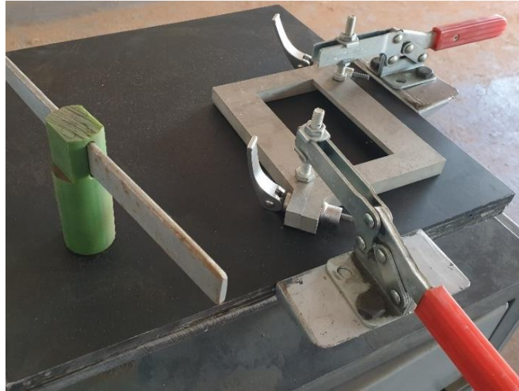
Figure 4.11: Casting-frame kept in place with toggle clamps
