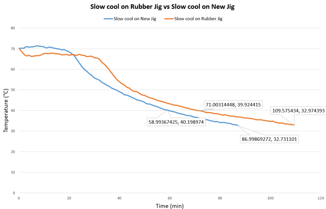
Figure 5.14: Cooling rate comparison between the commercial rubber jig and the new jig
