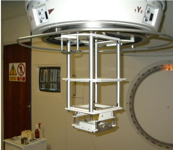
Figure 3.5: Elekta electron applicator at the National Hospital
