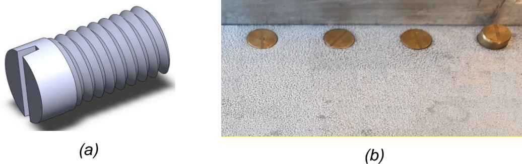
Figure 4.20: (a) CAD blank of M8 binary pin and (b) binary pins screwed into base
