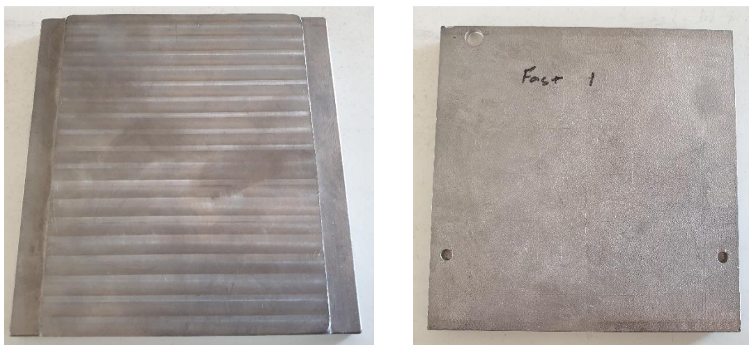
Figure 5.17: Top and bottom surface of a fast-cooled end-frame cast on the new jig
