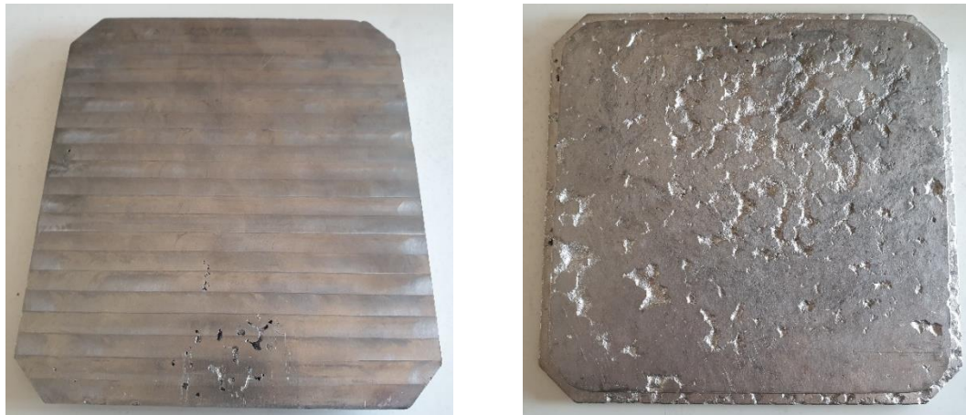
Figure 5.16: Top and bottom surface of an end-frame cast on the commercial jig showing cavities
