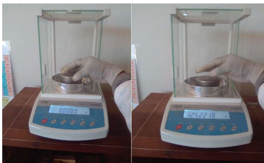
Figure 4.31: Moisture tin is weighed before filter papers were taken out from the jar.
