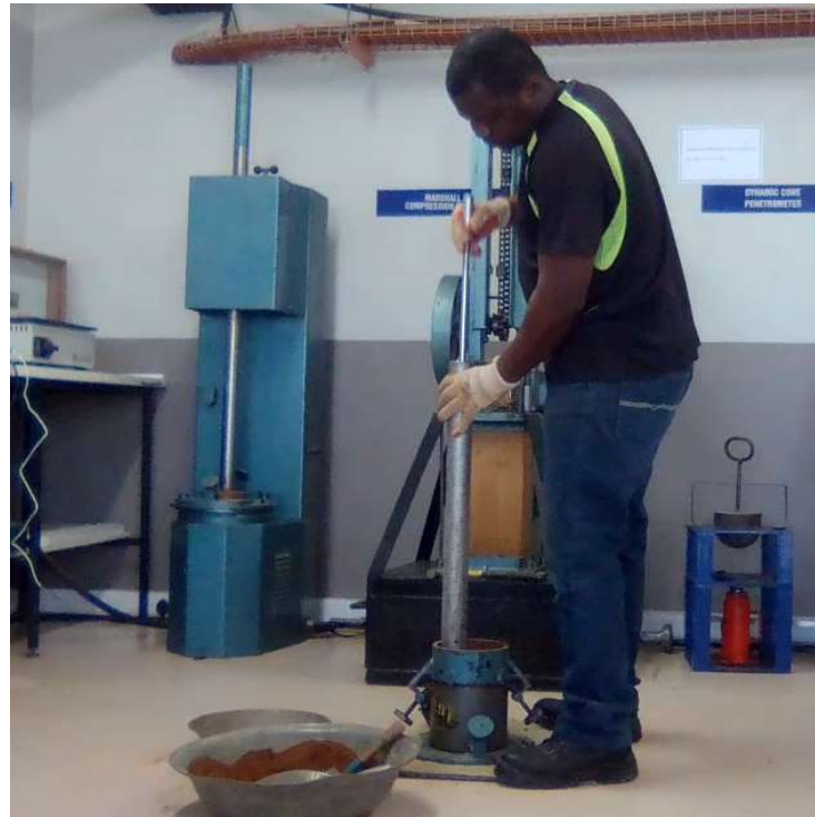
Figure 4.15: Proctor compaction test
