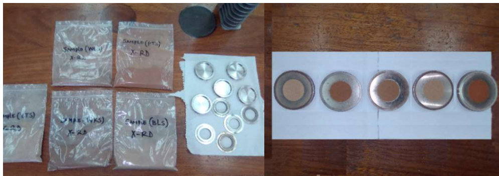
Figure 4.12: Sample preparation by front-loading for XRD test
