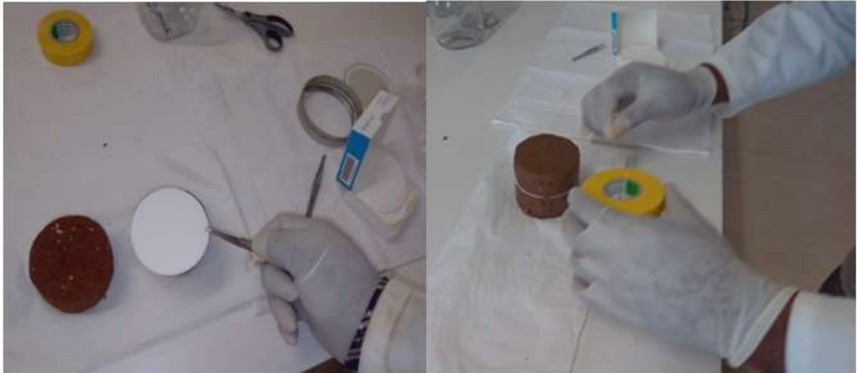
Figure 4.27: Three filter papers placed for matric suction measurement.
