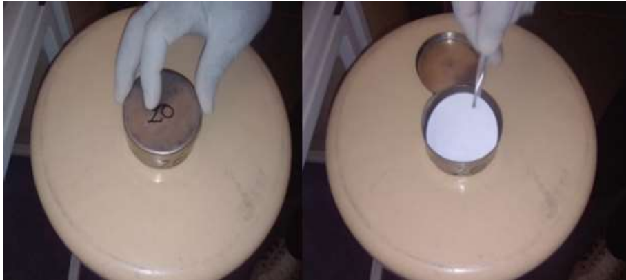
Figure 4.32: Filter paper put into labeled moisture tine for suction measurement.
