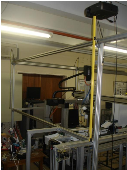
Figure 4.21 Light curtains mounted on the sides of the Cartesian robot
