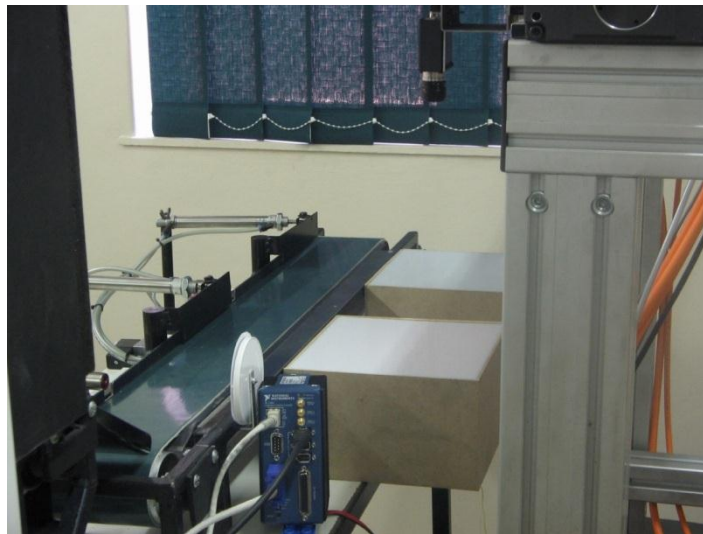
Figure 5.7 Two light boxes with 50W halogen lamps
