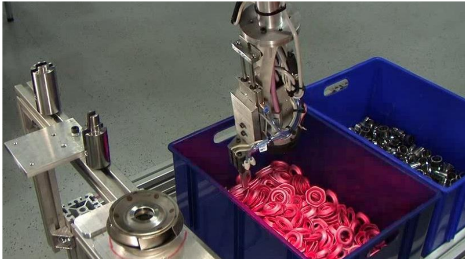
Figure 2.28 Kuka robot used for bin picking [61]
