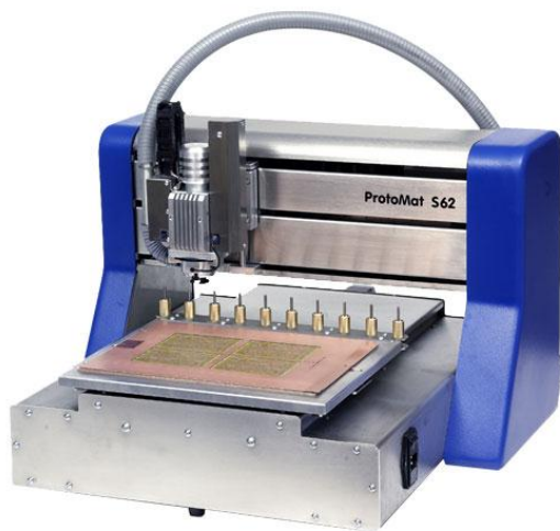
Figure 2.6 Circuit board plotter [24]
