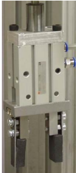
Figure 3.17 Parallel fingers designed for the pneumatic cylinder
