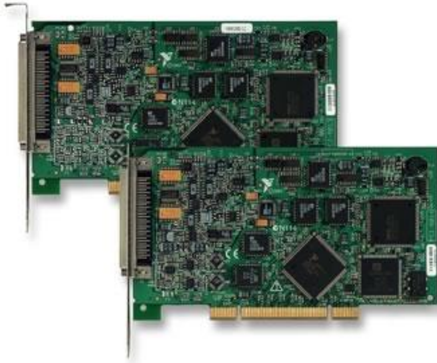
Figure 3.4 NI PCI 6014 Data Acquisition card [63]
