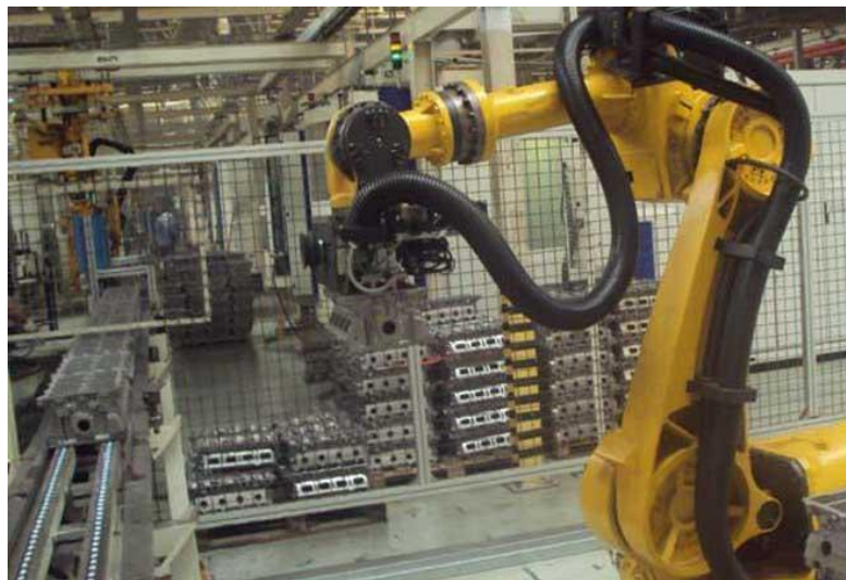
Figure 6.1 Smart camera and robot integrated to pick cast parts from a pallet onto a conveyor [86]
