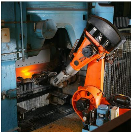
Figure 2.4 A Pick and Place robot in a factory [17]
