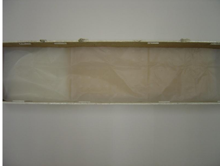
Figure 5.12 Diffuser placed over the LED array
