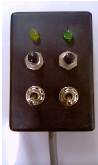
Figure 3.7 PLC simulator switch unit
