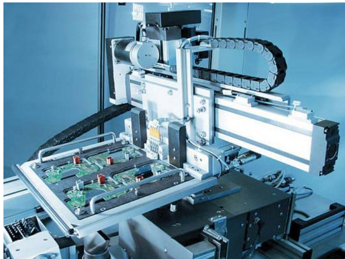
Figure 2.8. Circuit breaker welding system [27]
