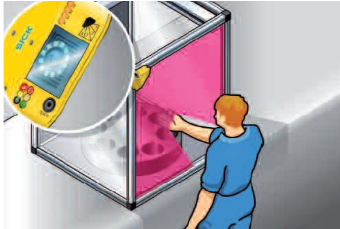
Figure 2.23 Hand detection safety systems [55]
