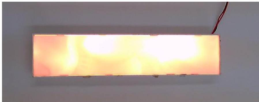
Figure 5.10 Bright spots on the inspection bay
