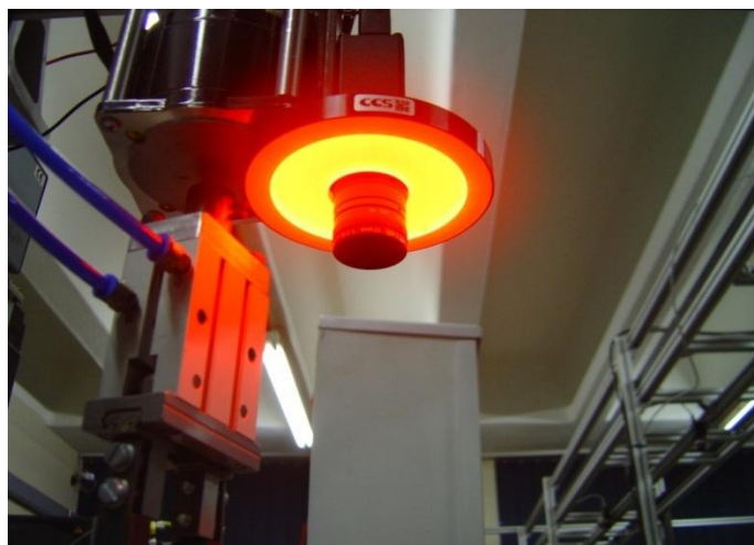
Figure 5.5 Diffused ring light mounted on Machine Vision camera
