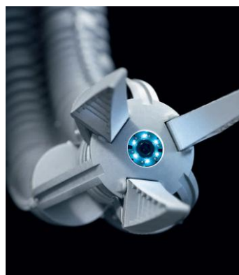
Figure 2.27 Adaptive gripper with integrated camera [58]
