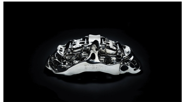
Fig. 9. Bugatti brake caliper – currently the world’s largest functional part produced in titanium alloy Ti6Al4V by AM – for the Bugatti Chiron vehicle. Example used with permission from Bugatti [84].
