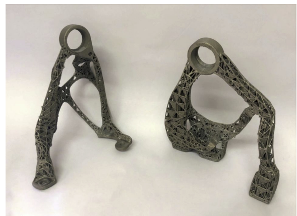
Fig. 18. Example of two topology optimized and latticed brackets produced by laser powder bed fusion in Ti6Al4V. These parts include internal supports in the lattice structure which cannot be removed. An improved design for the lattice is required to ensure no supports are needed inside the lattice regions.
