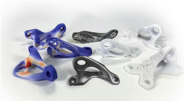
Fig. 20. Combining topology and lattice optimization into one simulation-driven design process results in “lattice struts” which have a curved geometry following load paths. Parts designed by ParaMatters [138], manufactured by 3D Systems and XPponentialWorks.
