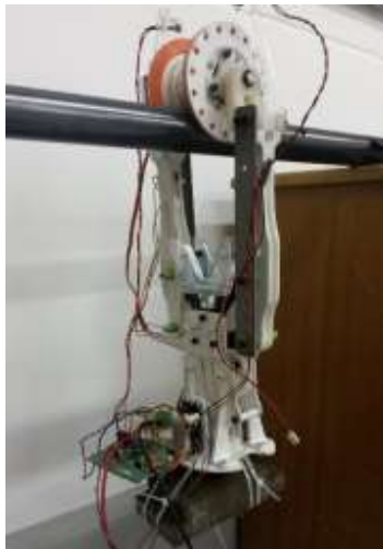
Figure 35 Brachiating robot gripper/pulley.
