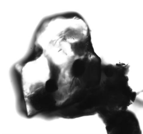
Figure 1. Coarse Sand layer from Heidedal soil, Test Pit 1 Layer 1 (TP1, LR1). Dispersant Sodium Hexametaphosphate and Sodium Carbonate.
