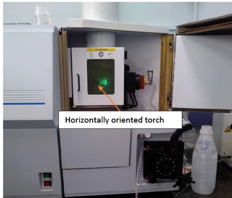
Figure 5.2: Prodigy 7, ICP-OES showing a horizontally oriented torch
