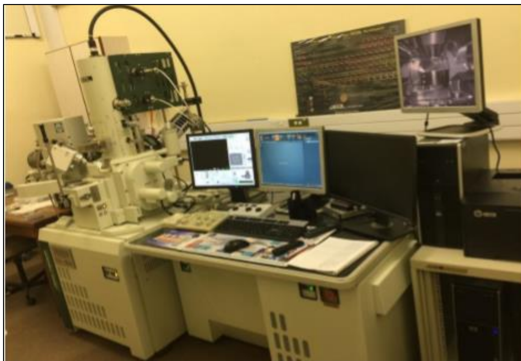
Figure 4.5: SEM instrument showing the electron column, sample chamber, Energy-dispersive X-ray spectroscopy (EDX) detector, electronics console and visual display monitors
