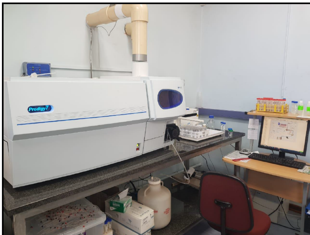
Figure 5.1: Prodigy 7, ICP-OES used in the determination of heavy metals in abattoir wastewater
