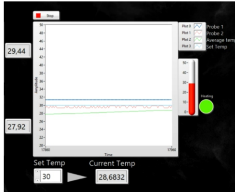
Figure 6: Software used to control calibration surface temperature
