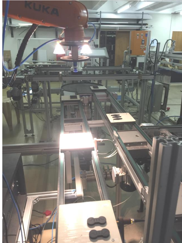
Figure 4-10 Component Conveyor - KUKA Robotic scans pallet to learn items
