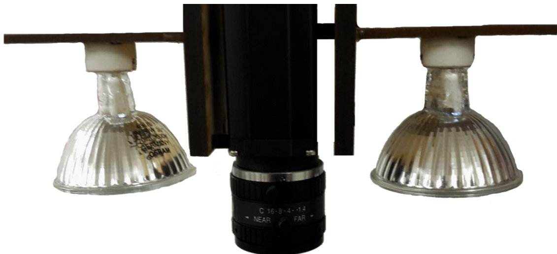
Figure 3-5 Example of the fixed lighting setup attached to the end effector
