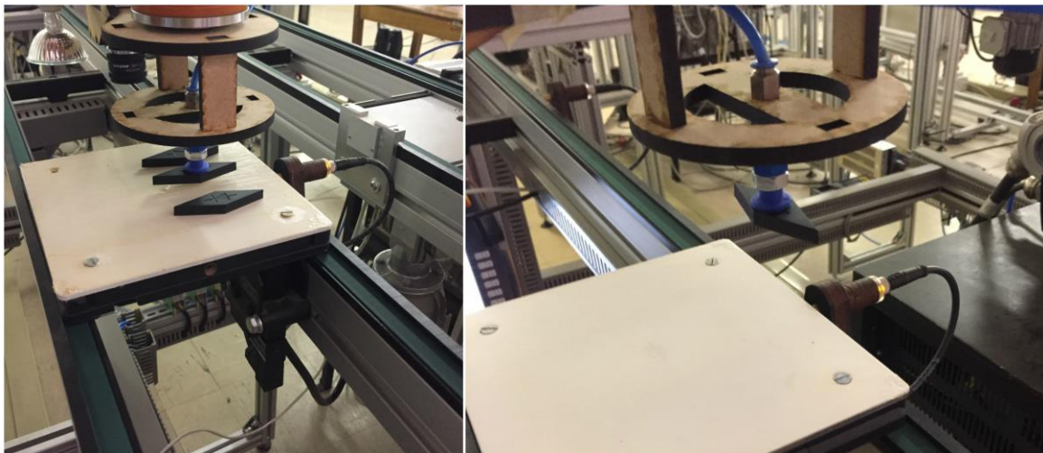
Figure 4-19 Example of the first component being picked up and placed on the design conveyor
