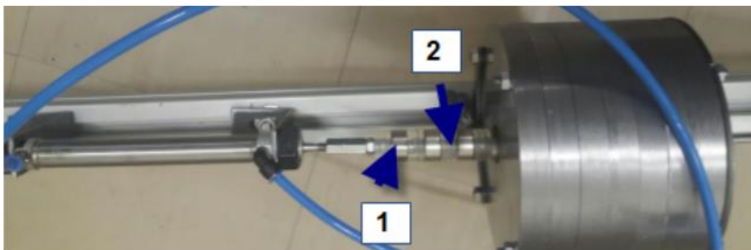
Figure 3.7: Side view of the Engine showing magnets and separators
