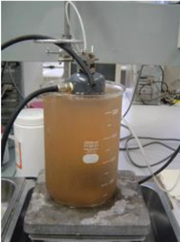
Figure 4. 10: Apparatus for aerobic screening during the grey water treatment process
