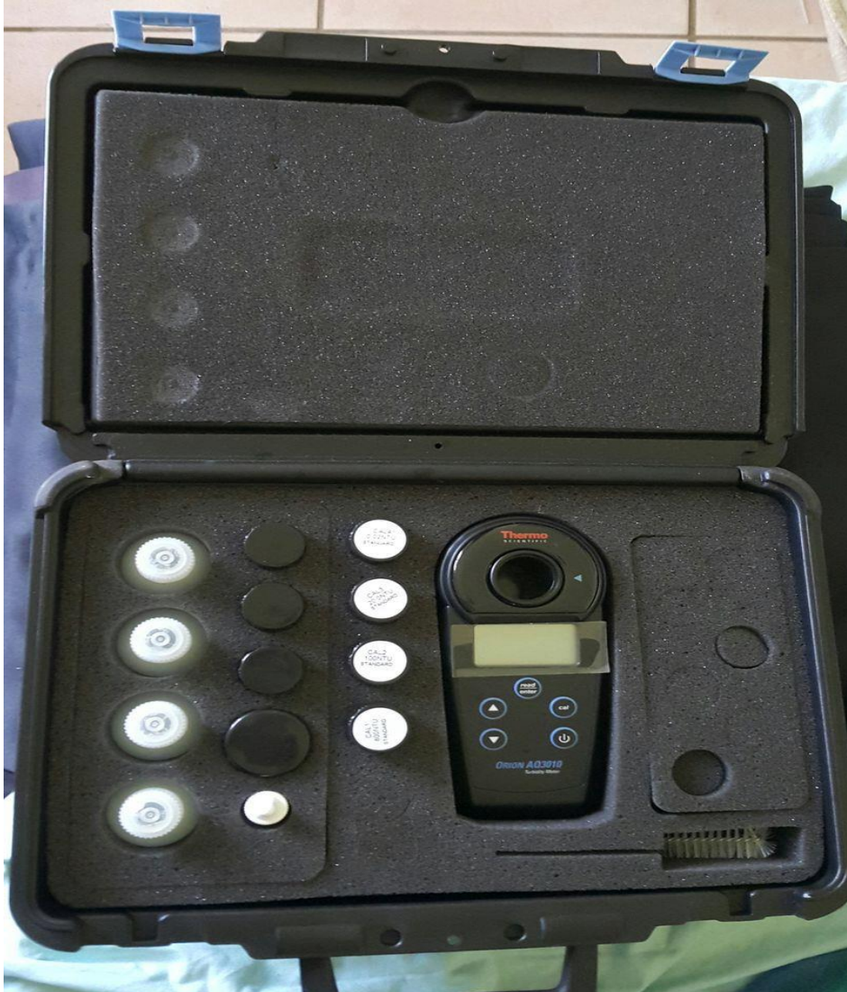
Figure 4. 15: A Turbidity meter for measuring the degree of cloudiness of grey water
