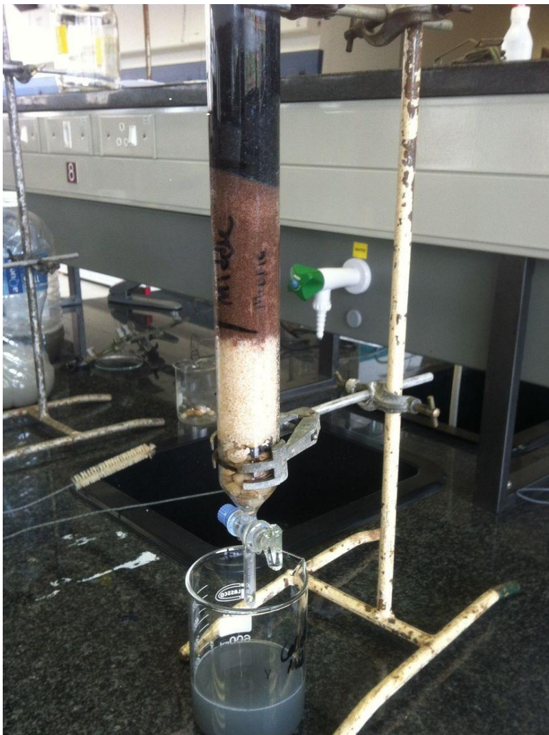
Figure 4.12: Multimedia filtration process
